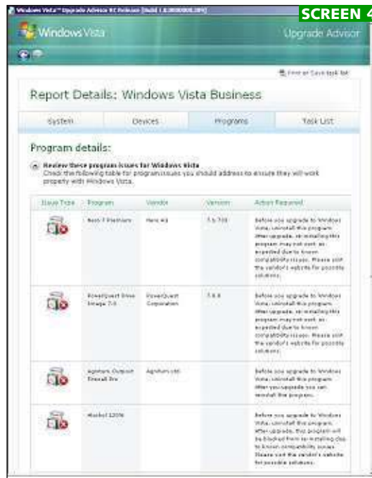
The Windows Upgrade Advisor checks whether or not your system is suitable for Vista
